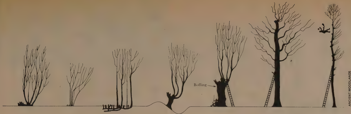
Methods of producing wood from trees. Left to right: coppice stool above ground (e.g. ash); coppice stool below ground (e.g. hazel); clone of suckers (e.g. elm); stub on boundary-bank; pollard; high pollard; shredded tree. The left-hand half of each has just been cut; the right-hand half is fully regenerated and is about to be cut again.
